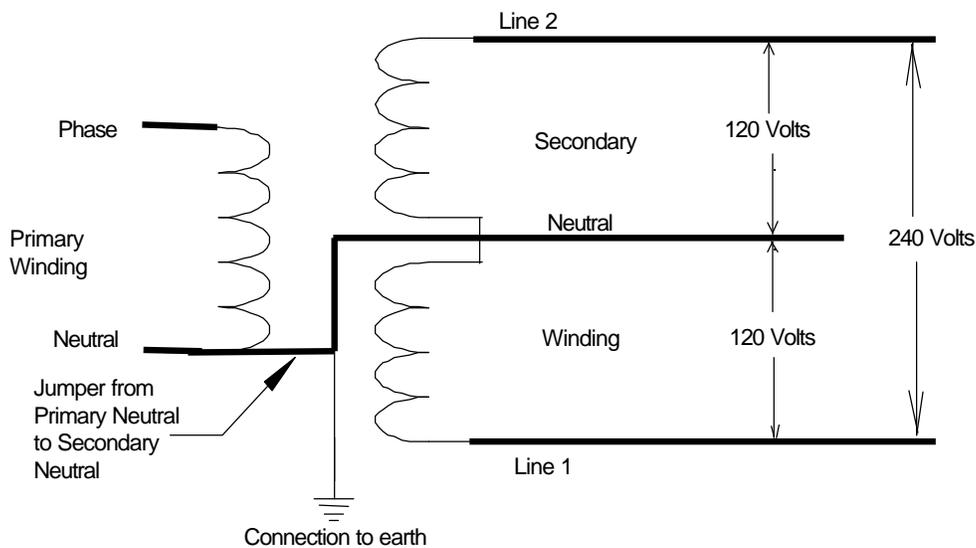
Figure 13. Phase to Neutral Primary Connection with Secondary winding Center Tapped and the Primary Neutral Connected to the Secondary Neutral.
