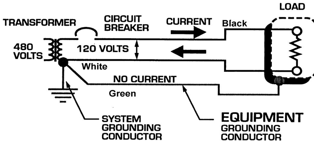
**Figure 1.** Circuit diagram showing the black phase conductor carrying current, the white neutral conductor carrying return current and the equipment grounding conductor carrying no continuous current.
