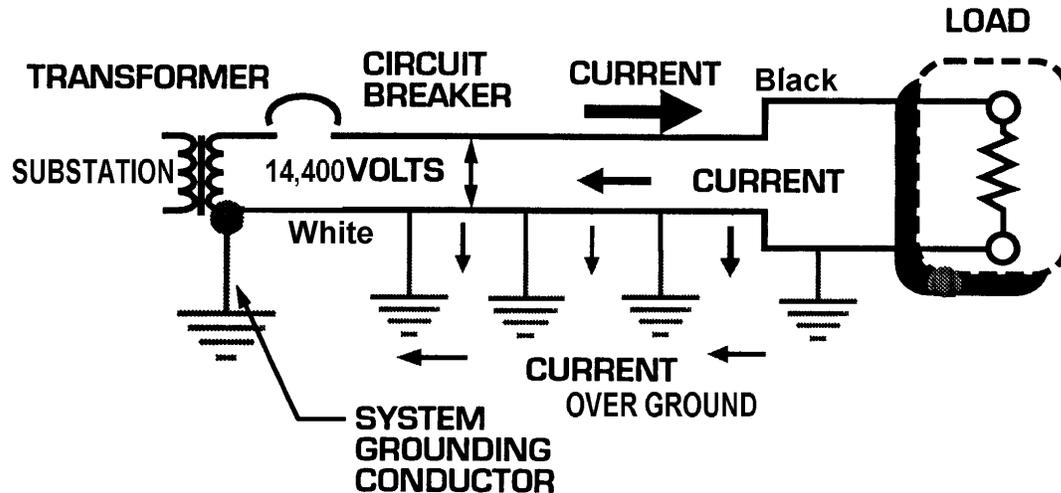
**Figure 2.** Diagram showing the electrical substation with a transformer, protective device, the circuit breaker, the two electrical distribution conductors, the multiple connections of the neutral to earth and the flow of uncontrolled electric current over the earth.
