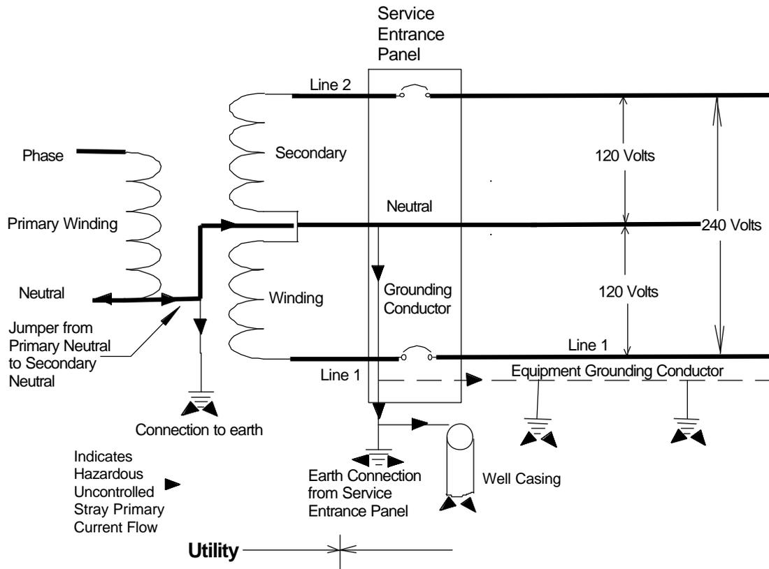
Figure. Wiring Diagram Showing the Hazardous Uncontrolled Stray Primary Current Flow over . . .PUBLIC
