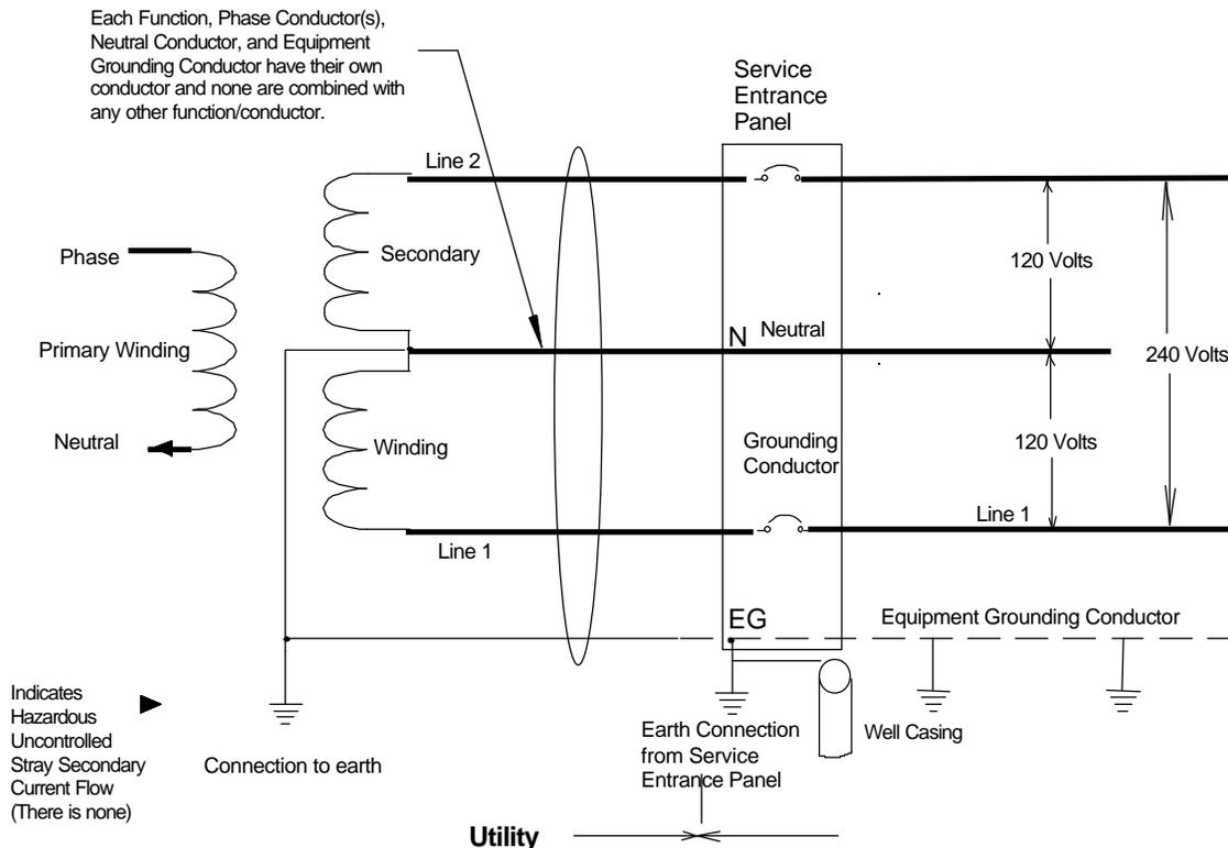
Figure 22. The Correct Number of Conductors for the Utilities Service Entrance
