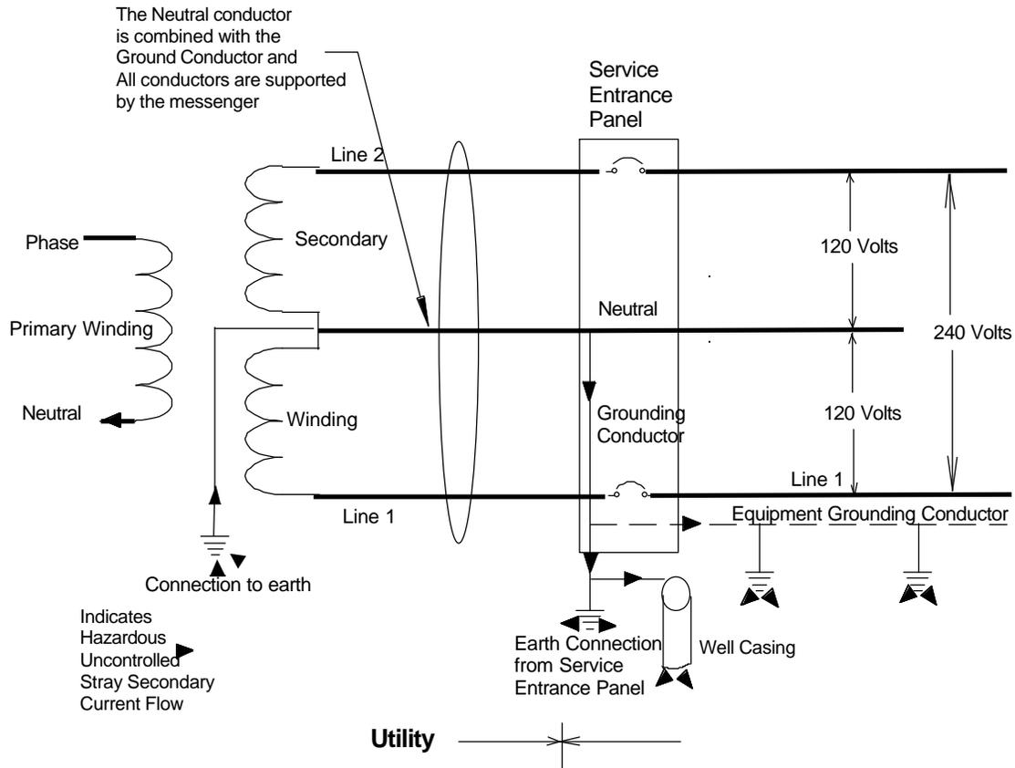
Figure. Conflict between the NESC and the NEC over the Grounding of the Neutral.
