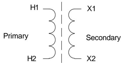
Figure 11. Transformer Electrical Isolated
